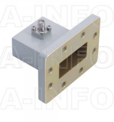
137WCAK Right Angle Rectangular Waveguide to Coaxial Adapter 5.85-8.2GHz WR137 to 2.92mm Female
